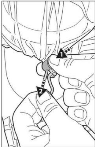
While holding the cord, press on the cord fastener and push it under the flange.
