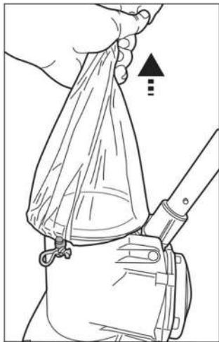
Lift up the bag to ensure it is totally secured before deploying the pool vacuum into water.
