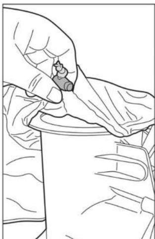
Spread the filter bag over the top opening of the main body of the pool vacuum. Make sure the cord of the bag is placed under the flange of the top opening.
